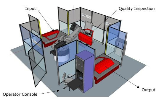
This fenced adaptive robot cell speeds up ultrasonic inspection and reduces measurement preparation time thanks to straightforward parts positioning and system calibration.
